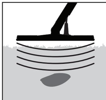
2. In the presence of the detector's electromagnetic field, eddy currents are induced in the metal target.
