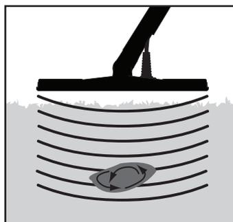
3. The eddy currents flowing within the target produce their own electromagnetic field, which is received by the metal detector's search coil.
